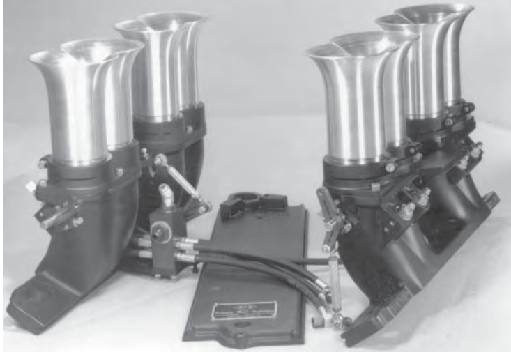
Constant flow fuel metering installed
