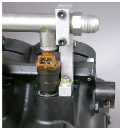
Stainless steel fuel rail, silver soldered for use with alcohol with special clamp mount
