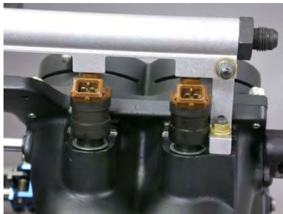
Aluminum fuel rail for use with gasoline with standard mount stanchion
