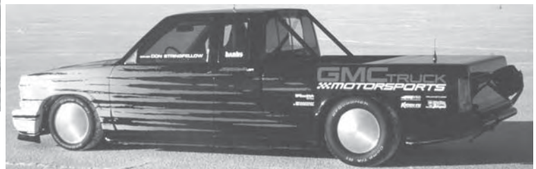
GMC Motorsport's S-15, the first truck to reach 200 MPH at Bonneville. Chevrolet 90° V6, engine built by Katech
