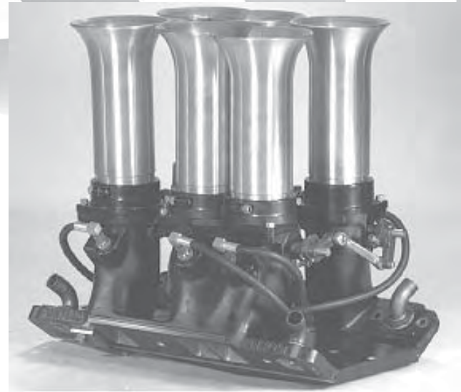
Constant flow metering
