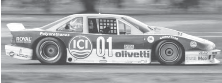
Trans-Am Champion: Chevrolet 90° V6, engine built by Katech. Kinsler manifold with EFI
