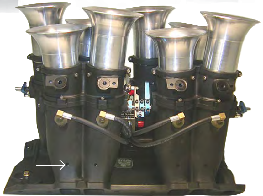
Traditional Kinsler big block Chevrolet manifold with optional 'low' nozzle location and nitrous nozzle ports
