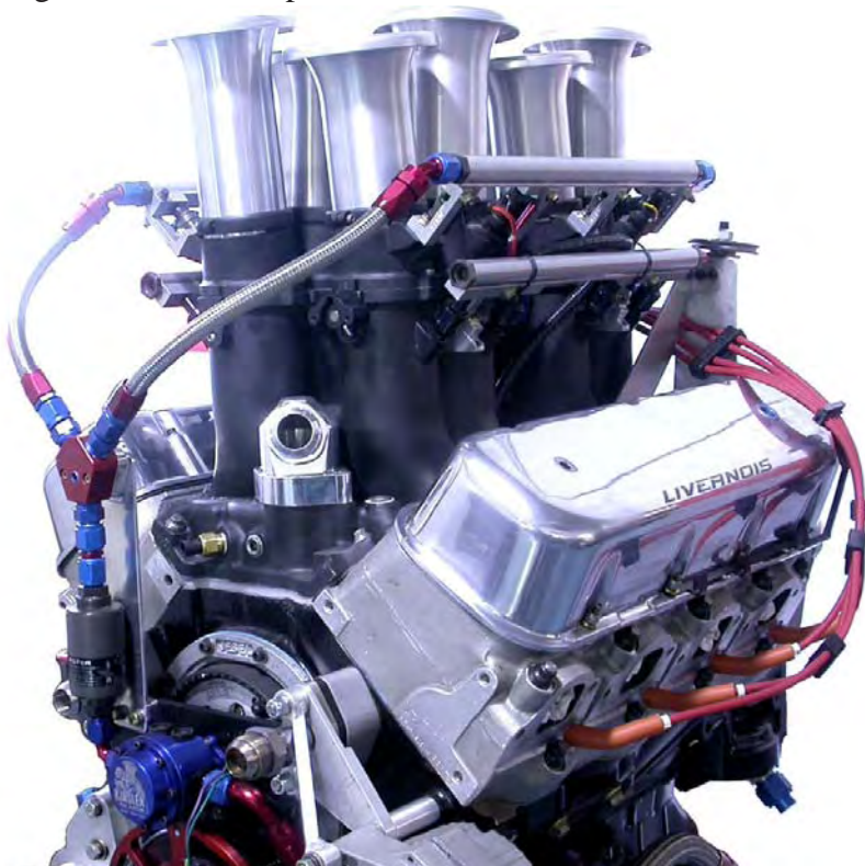
John Lohone's EFI big block Chevrolet. Note the mechanical fuel pump and 'lower' rail system for vacuum reference
