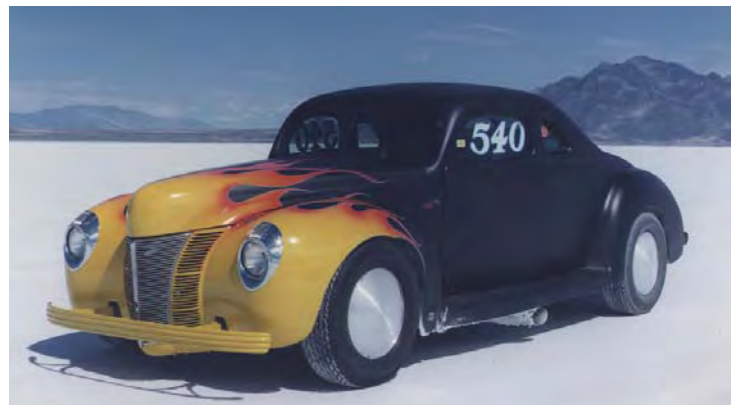
Jerry Helwig's Land Speed 1940 Ford Coupe powered by Kinsler injected flat head Ford, runs in XF/VGC on gasoline and XF/VFC with alcohol/nitromethance mixture
