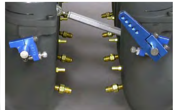
Manifold runners machined for M.A.P. reference (upper fitting) and I.A.C. (lower fitting) kits
