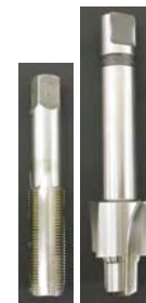
Closeup of 8 AN + o-ring thread detail
