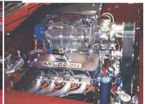
Kinsler Vapor Separator Tank and Jet Selector Valve mounted in lower right corner of the photo
