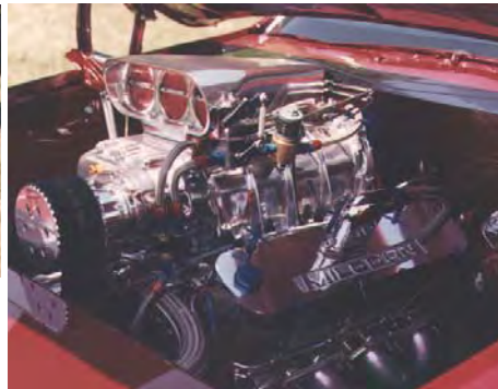
Kinsler SS-12 Electric Fuel Shut-off valve mounted near the barrel valve on the blower hat
