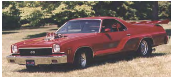
Al Mullin's Pro-Street 468 CID big block Chev El Camino. 6-71 supercharger on gas using Kinsler constant flow system
