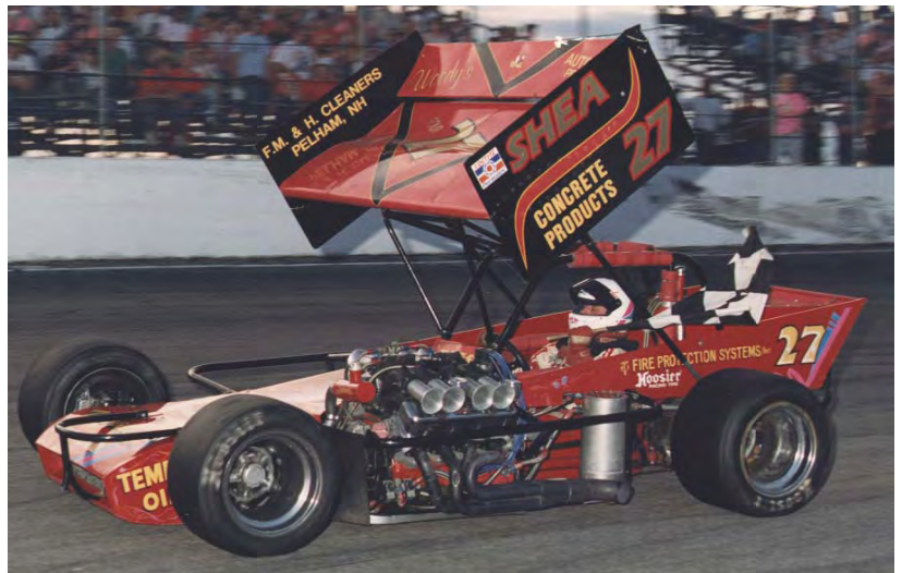
Eddie Shea's Super Modified uses a Kinsler cross-ram manifold with constant flow system on a big block Chev
