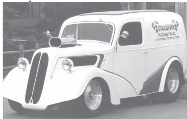
Chris Cherry's 'Pro-Street' Thames panel van. Kinsler modified Hilborn 4-port blower hat on a 6-71 supercharged small block Chev on gas. Uses a Kinsler Jet Selector Valve and Vapor Separator Tank.
