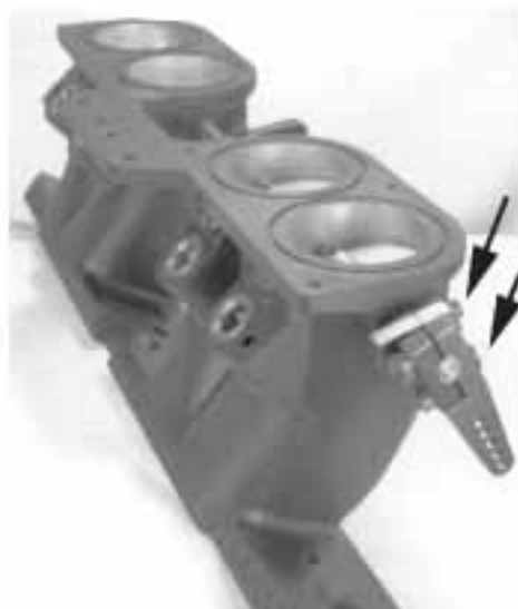
CORRECT Pulling arm installed next to throttle stop
