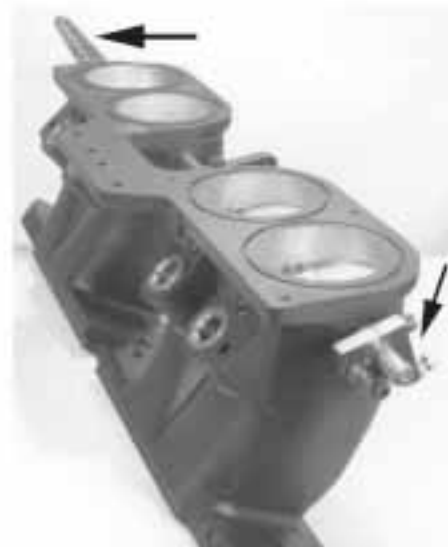
!!! INCORRECT!!! Pulling arm on the opposite end of the manifold from the throttle stop
