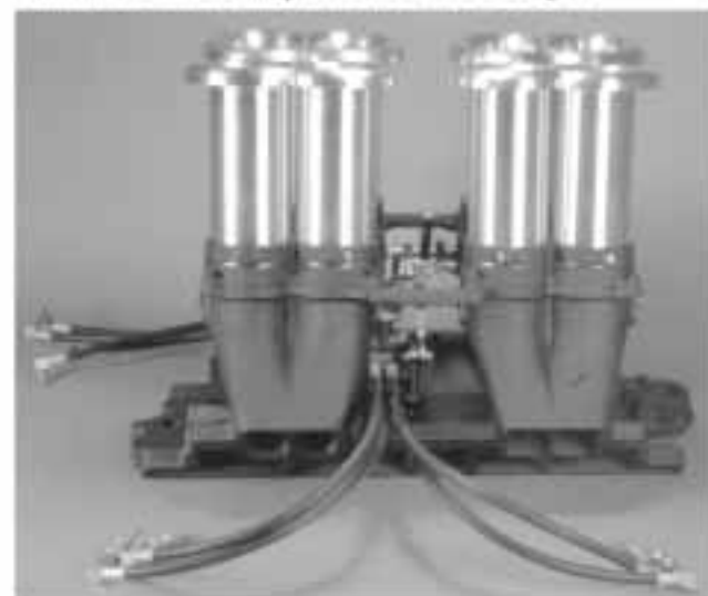
'XTRA LIGHT' 2 5/8" throttle size manifold. Nozzle bosses removed from castings. Optional port profile: All Pro 285 Stage II
