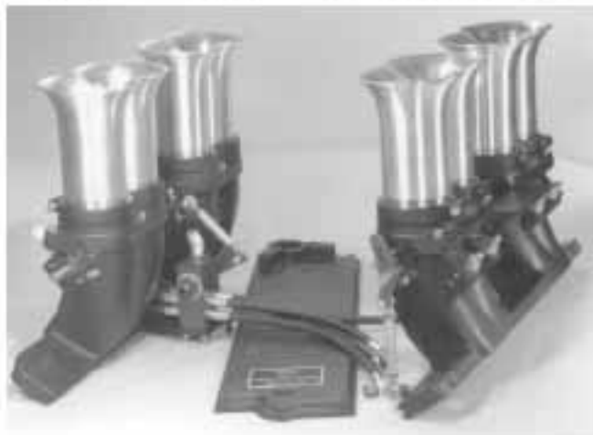
Constant flow fuel metering installed
