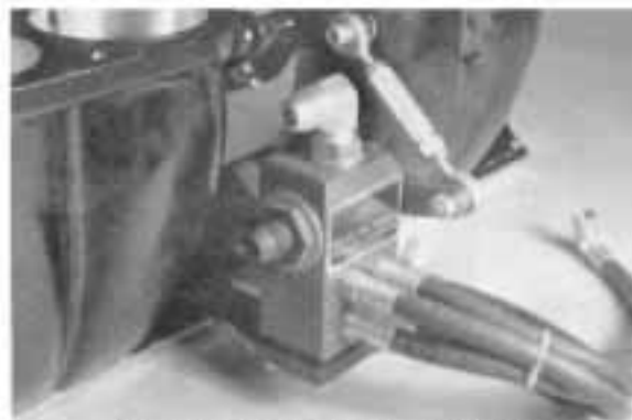
Barrel valve mounted to a bracket attached to the manifold. This keeps the barrel valve off the hot valley plate.
